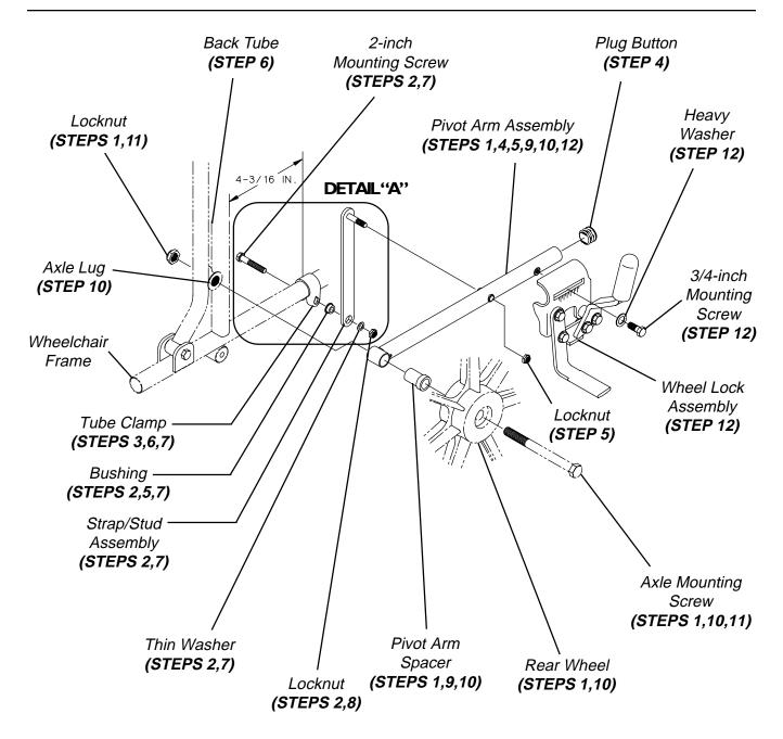
FIGURE I-REPLACING THE PATIENT OPERATED WHEELLOCKS
